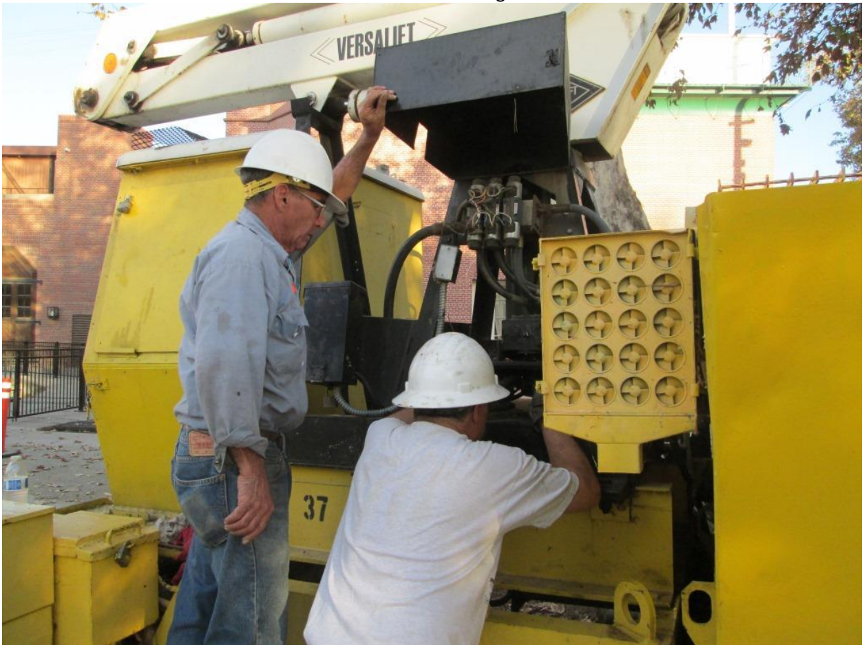
Mike T. and Mike H. work on the gear-box of the man-lift
