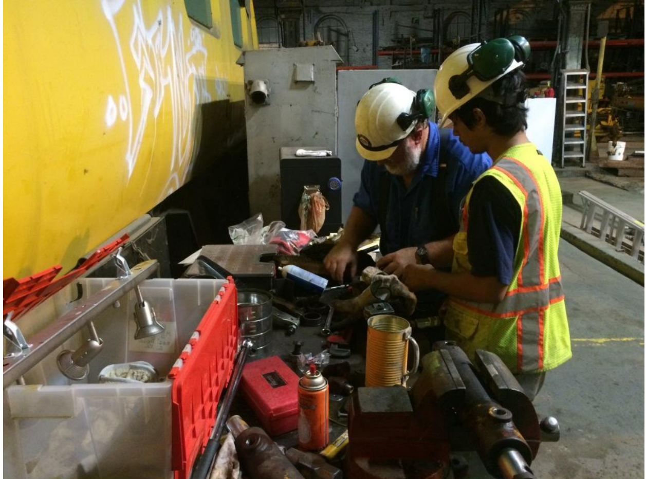
Frank and Josh removing the hydraulic fitting from the squeeze cylinder of the secondary section-gang machine
