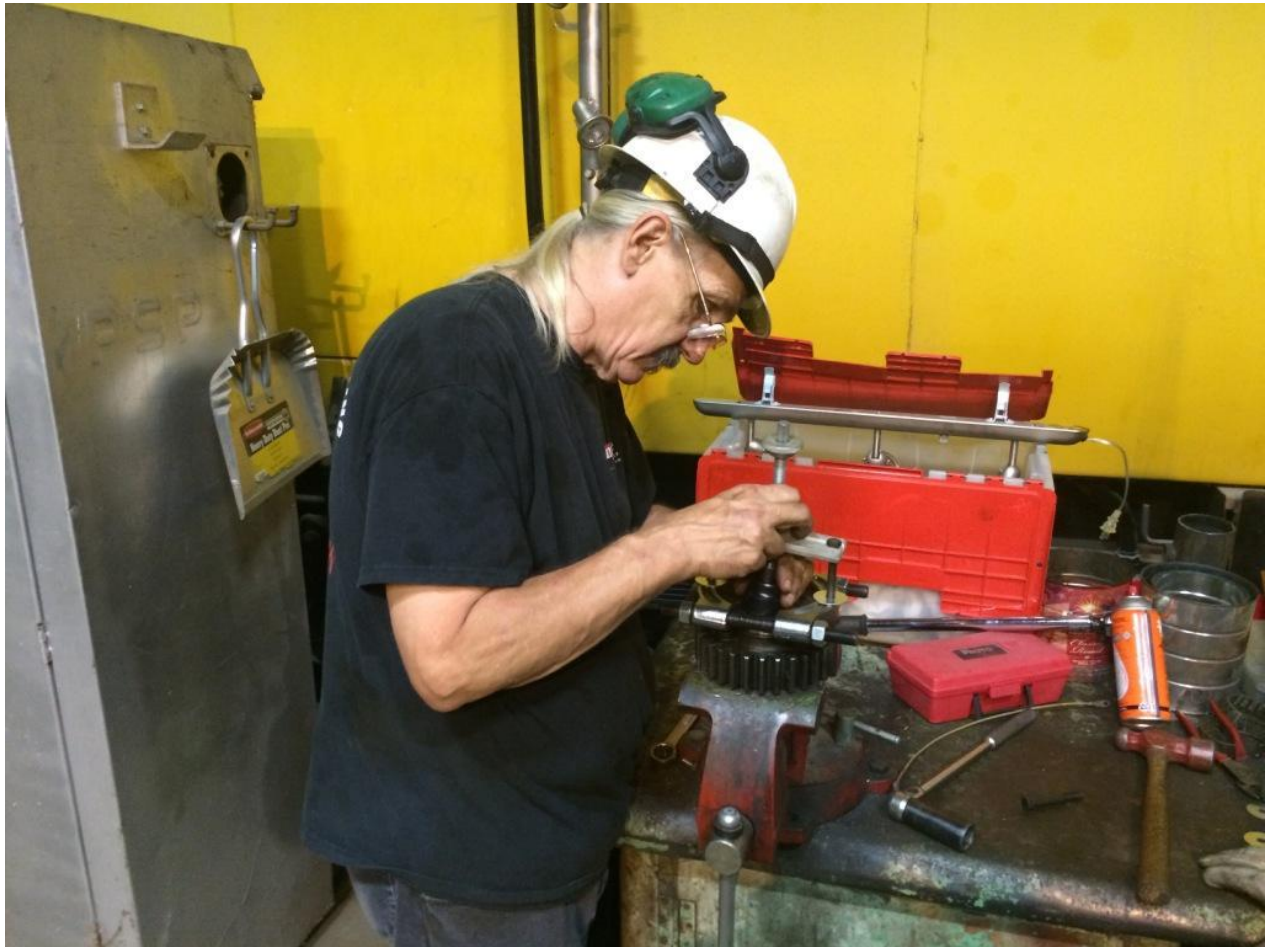
Fred pulling the bearing from a gear out of the tie-shear's dual drive
